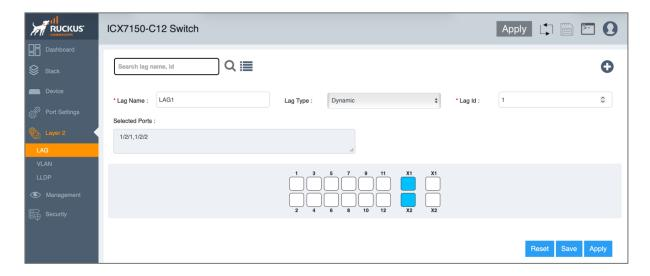
RIVI switches support up to 128 LAG groups, each with up to 16 member ports. Create multiple LAG groups only if you need to separate traffic by VLAN or require multiple switch-to-switch connections.
