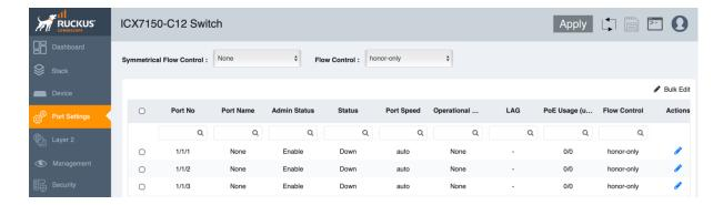
The **Port Settings** menu is used to edit the configuration of ports individually.
