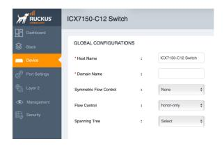
The **Device** menu is for Global Configuration of the switch and used to set the Host Name and (optionally) Domain Name of the switch.
