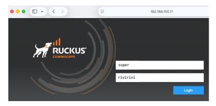
**IMPORTANT:** Switches that are in a factory reset condition have the username **super** and password **sp-admin**. After these credentials have been used the first time you will be prompted to change the password.
